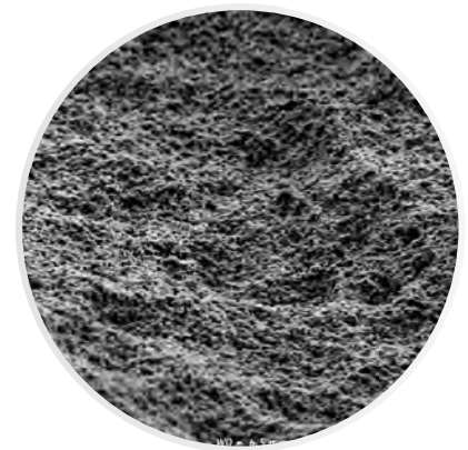
Representative image of the implant surface - Scanning Electron Microscope (SEM) magnification of 5000x.
